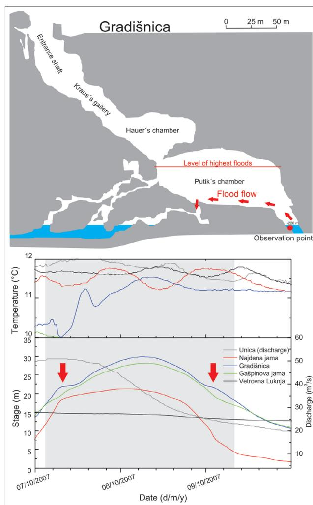
**Figure 7:** a) Simplified cross-section of Gradišnica adapted from NAGODE (1997) with the position of the observation point and assumed flow direction at high floods. b) Detail of Event 3 with the inflection in the stage hydrograph, which occurs when the Putick's chamber is filled and emptied.
