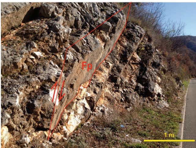
Figure 7. Photograph of the reverse fault plane (Fp=24/62) in the recrystallized limestones of the Gornji Humac fm. along the NE margin of the Vinodol Valley. Location: 45°16'15.5"N, 14°36'14.2"E.
