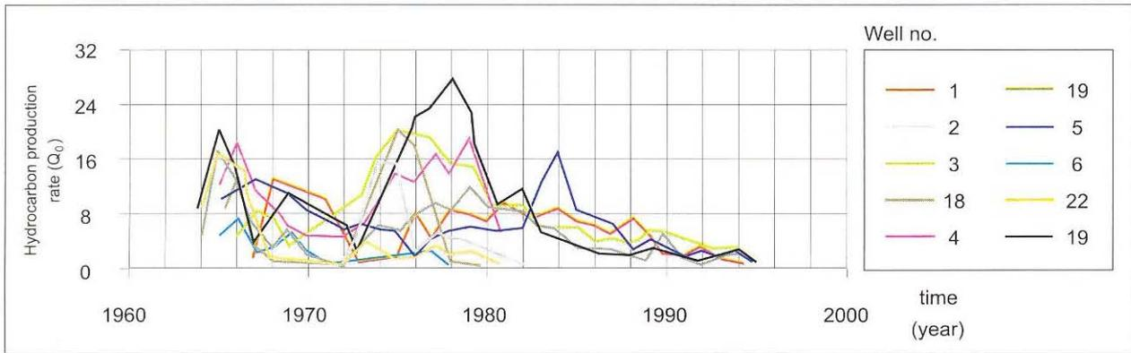
Fig. 3 Hydrocarbon production rate - “bad producers”.
