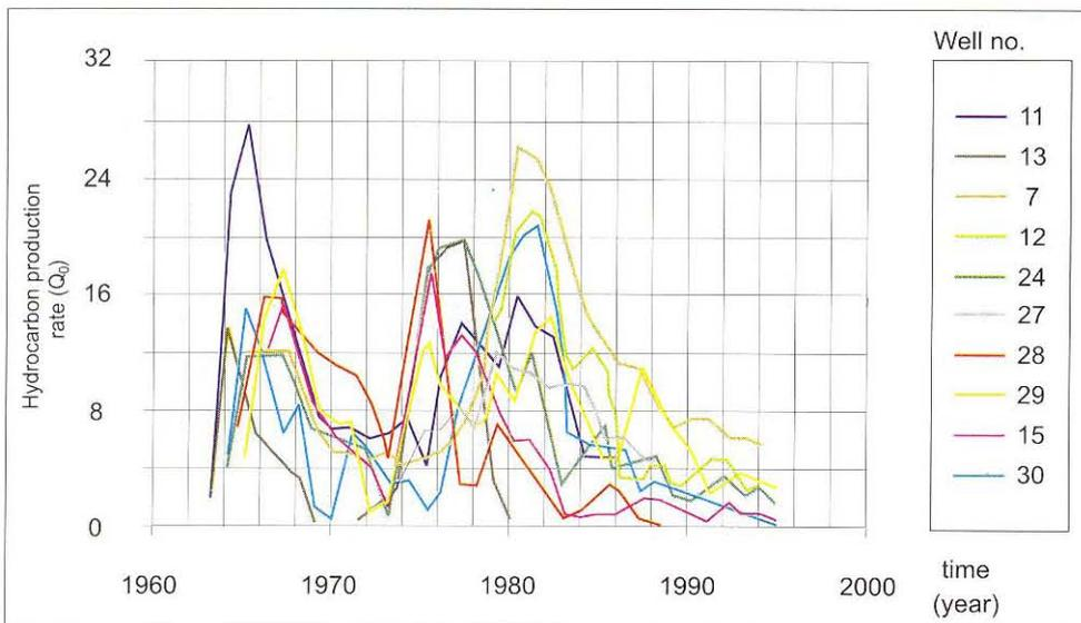
Fig. 4 Hydrocarbon production rate - “good producers”.
