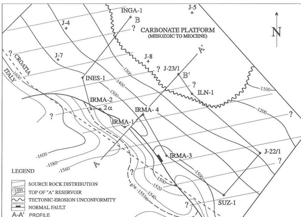
Fig. 2 Structural contour map of the top of the "A" reservoir (after KADIJA et al., 1991) of the Irma gas field with distribution of the source rocks overlying the top of the reservoir (profile B-B').
