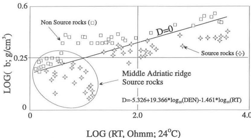
Fig. 11 Bulk density vs. resistivity crossplot plotted on the logarithmic scale. The oblique line is the position of D=0 (Discriminant analysis). Points below this line (D=positive: star) = source rocks; points above this line (D=negative: rectangle) = non source rock. The analyses are from an area of the Middle Adriatic ridge, Sava and Drava depression (after VULAMA, 1994).
