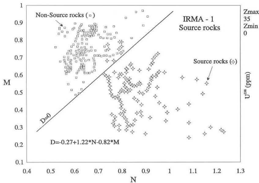
Fig. 19 M/N(Z) four component crossplot consisting of a combination of sonic transit time, bulk density, compensated neutron porosity and  $Z=U^{238}$ . The oblique line is the position of  $D=0$  (Discriminant analysis). Points below this line ( $D$ =positive: star) = source rocks; points above this line ( $D$ =negative: rectangle) = non source rock. The analysis is from IRMA-1 well (Middle Adriatic ridge).
