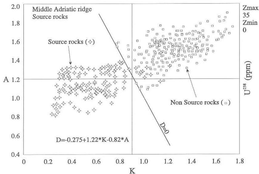
Fig. 14  $A/K(Z)$  four component crossplot comprising combination of sonic transit time, bulk density, compensated neutron porosity and  $Z=U^{238}$ . The oblique line is the position of  $D=0$  (Discriminant analysis). Points below this line ( $D$ =positive: star) = source rocks; points above this line ( $D$ =negative: rectangle) = non source rock. The analysis is from an area of the Middle Adriatic ridge.
