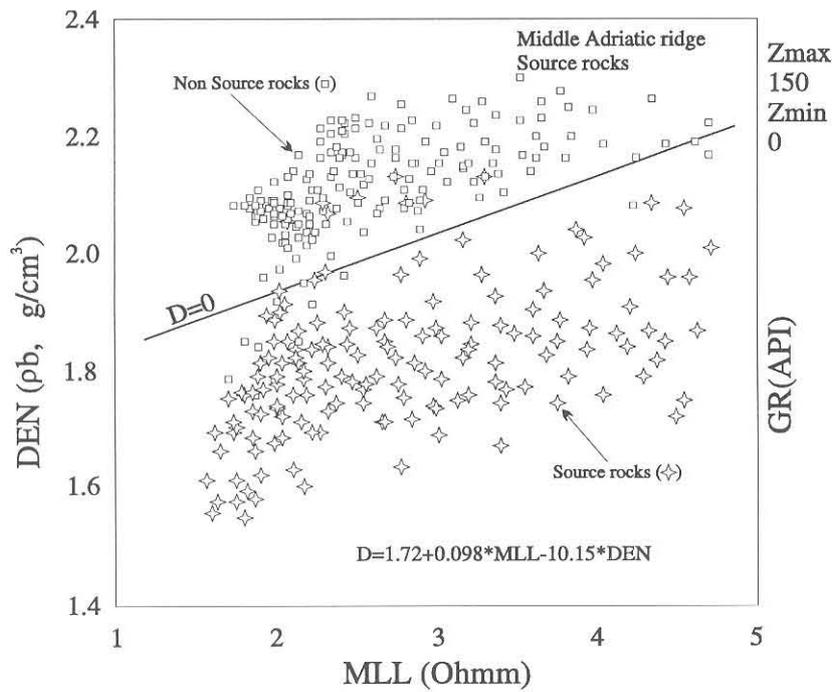
Fig. 12 Bulk density vs. resistivity crossplot plotted on the linear scale. The oblique line is the position of  $D=0$  (Discriminant analysis). Points below this line ( $D$ =positive: star) = source rocks; points above this line ( $D$ =negative: rectangle) = non source rock. The analysis is from an area of the Middle Adriatic ridge.
