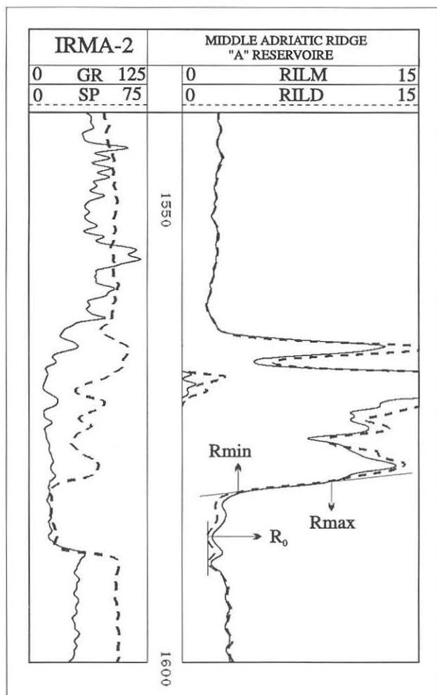
Fig. 18 Permeability estimation from resistivity gradient in Miocene reservoir rocks of the Irma gas field (a consistent result with laboratory analysis).
