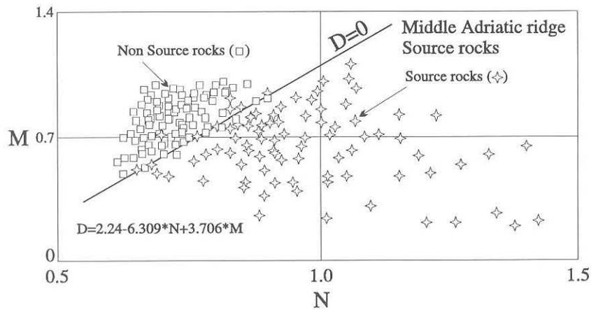
Fig. 13  $M/N(Z)$  four component crossplot consisting of a combination of sonic transit time, bulk density, compensated neutron porosity and  $Z=U^{238}$ . The oblique line is the position of  $D=0$  (Discriminant analysis). Points below this line ( $D$ =positive: star) = source rocks; points above this line ( $D$ =negative: rectangle) = non source rock. The analyses are from an area of the Middle Adriatic ridge (after VULAMA, 1994).
