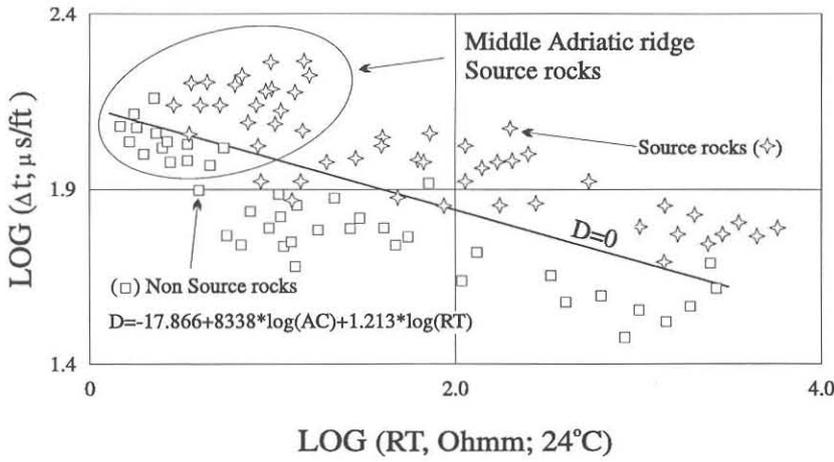
Fig. 9 Sonic transit time vs. resistivity crossplot plotted on logarithmic scale. The oblique line is the position of D=0 (Discriminant analysis). Points above this line (D=positive: star) = source rocks; points below this line (D=negative: rectangle) = non source rock. The analyses are from an area of the Middle Adriatic ridge, Sava and Drava depression (after VULAMA, 1994).
