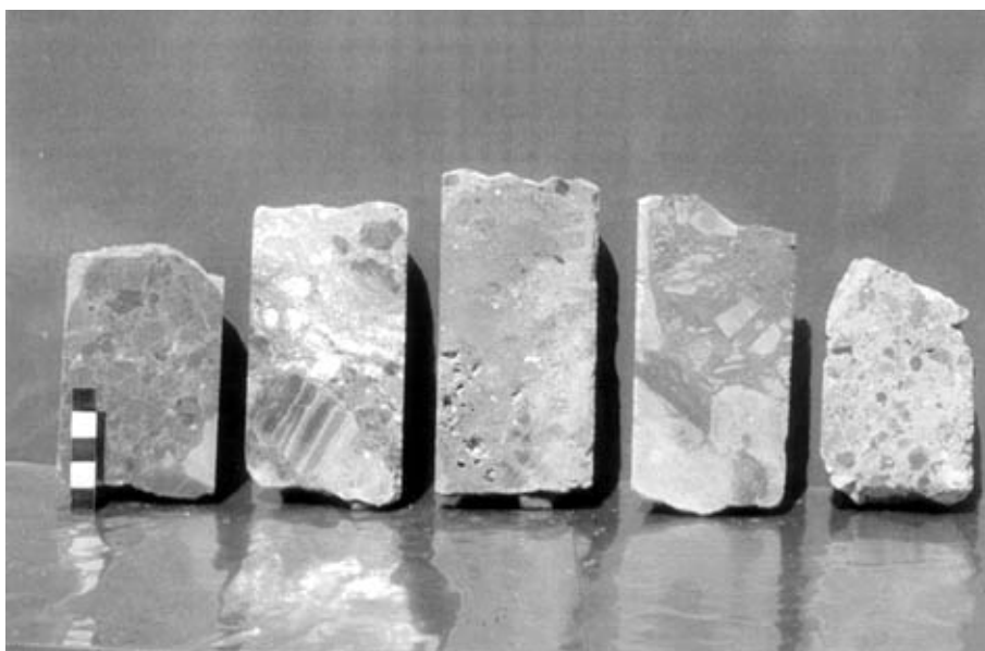
Fig. 9 Five typical examples of different varieties of the studied breccia from well ŽTC-2. A) Completely corroded dolomite fragments ("rounded" grains) surrounded by a large quantity of finely crushed recrystallized matrix; B) Large fragments of dolomite "floating" in dark calcitic matrix; C) matrix-rich breccia characterised by intense corrosion (isometric solution vugs formed by dedolomitization); D) breccia composed of completely silicified white fragments and laminated early-diagenetic dolomites; E) fractured dolomite with thin fillings of white calcite between dolomite fragments.
