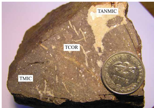
Figure 17: White coarse grained ankerite (sample TANMIC) occurs in the form of an irregular nest in a matrix of reddish coarse grained siderite (sample TCOR) which is surrounded by dark fine grained siderite (sample TMIC).
