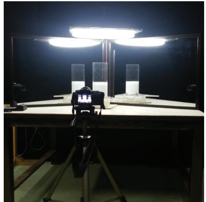
Figure 3. Digital image acquisition experiment setup.
