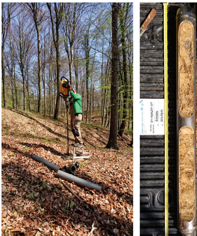
Figure 8. In-situ coring with the Atlas Copco Cobra system and corresponding core. The recovered cores are 100 mm in diameter.
